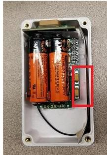
5. After replacing the batteries a brief led will turn on to indicate the device is powered up.
