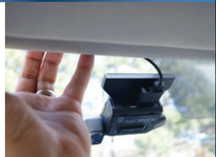
Route the cable along your windshield frame, ensure the cable is tucked alongside existing wires of the pillar and behind pillar air bag.
