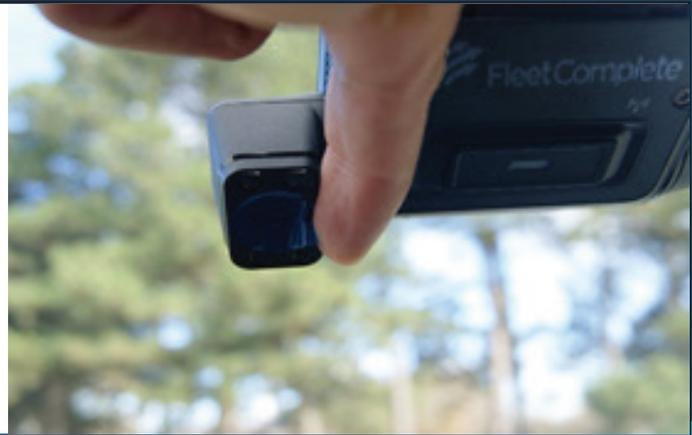
Using the allen key loosen the Camera lens screws so you can adjust your lens positioning. Fasten your screws only once you have completed the Vision Camera Alignment in page 7.
