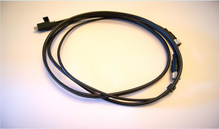
Connect your Micro USB cable end to the Camera next, connect your 6 pin M8 male receptacle end to the OBD to M8 female receptacle in image.
