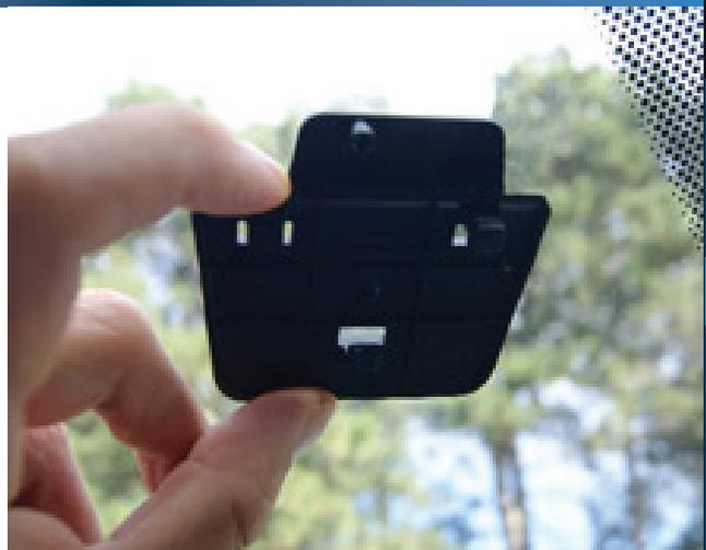
Attach the camera to the rear plate by matching the positions of the three mounting holes on the back of the camera with the hook on the rear plate. Slide the camera to the left to lock it in place.
