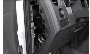
7. Mount the device in a location with least amount of exposure to damage by people or objects. Possible mounting locations are under the central console, behind the dash or behind the glove compartment.
